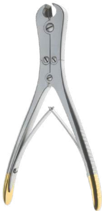
EKN6555 POWER TC 180 mm, 7 1 / 8 " wire: for 2,0 mm soft wire, hard 1,5 mm
